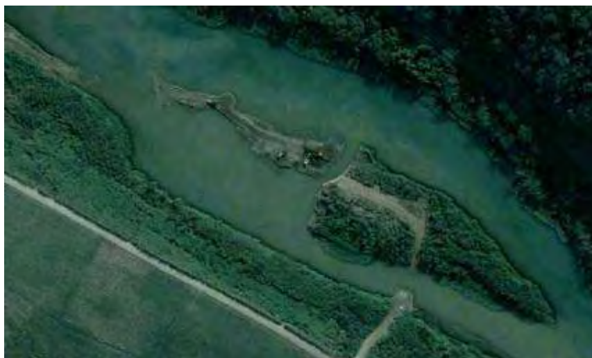
Figure 8.11 Example of estuarine sand mining operations in the Mzimkulu Estuary - note the sediment plumes (Source: Google Earth).
