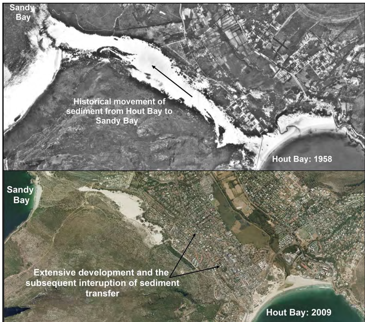
Figure 15: Historic sediment by-pass system in Hout Bay
